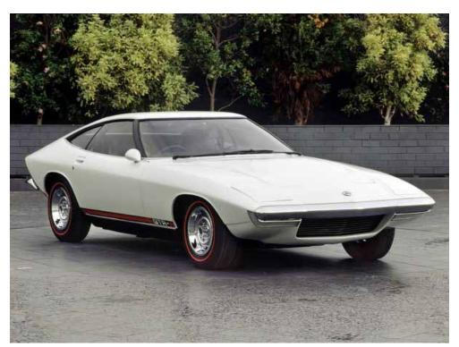
The GTR-X was produced by Holden in 1970 and was a three door hatch back coupe with a wedge-shaped fiberglass body. The prototype car had LC Torana GTR XU-1 mechanical components.
