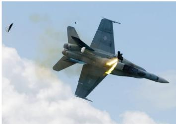
The white thing is the seat-stabilizing drogue chute. Notice the pilot's head pinned to his chest from the severe "g" forces produced by the solid rocket motors in the ACES II seat. They burn for about 2/10ths of a second ... Enough time to propel him at least 60 feet clear of the aircraft. One Hellova ride.
