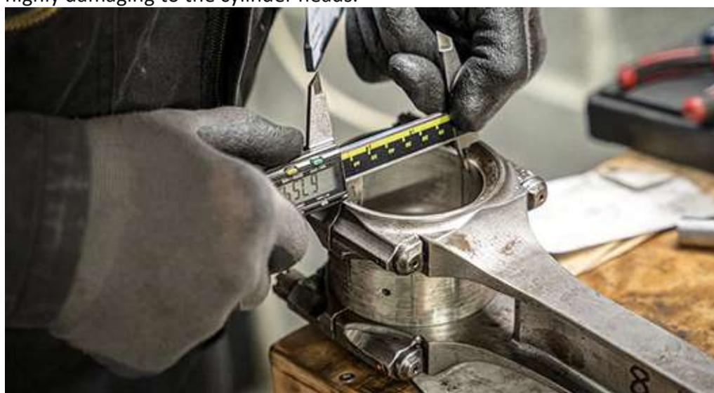
Con rod dimensions being measured to check the clearance on the bearings.
